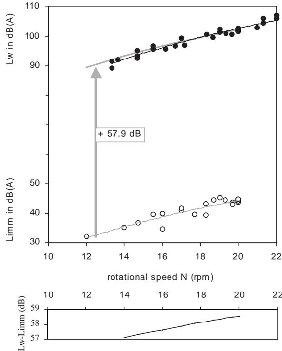
Fig. 7. Turbine sound power levels  $L_w$  measured near wind turbines (●) and immission levels  $L_{imm}$  measured at 400 m from wind park (○): averages differ 57.9 dB; (below) increase of difference  $L_w - L_{imm}$  with rotational speed.
