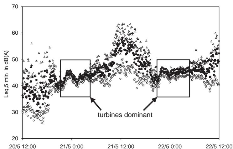
Fig. 4. 48 h registration of immission level ( $L_5 = \Delta$ ;  $L_{eq} = \bullet$ ;  $L_{95} = \circ$ ) per 5 min at location A; turbines are considered the dominant sound source if  $L_5 - L_{95} \leq 4$  dB.
